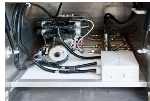
Hydraulikeinheit, Pop-Out/Pop-Up Wohnraum, Sattelschrank-Lift und Laderampen hydraulisch Hydraulic unit, pop-out/pop-up living quarters, hydraulic saddle compartment lift and loading ramps
