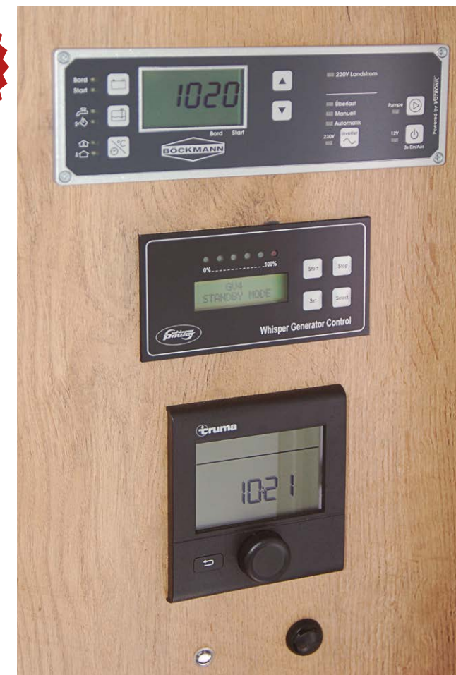
Bedieneinheit für Elektro, Heizung, Warmwasser, Klimaanlage, Generator, Hydraulik Control for electrical system, heating, hot water, air conditioning, generator, hydraulics
