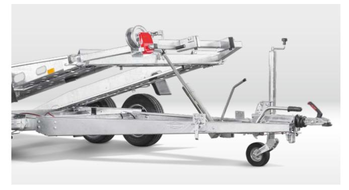
**Hydraulic lifting system and cable winch** Solid winch block with multi-position cable winch (AH and AT series).
