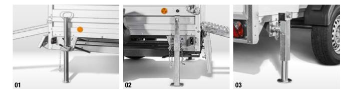
Safety supports (UT series only) Choose between sliding supports (01), reinforced sliding supports (02) or swivelling and extending telescopic crank supports (03).
