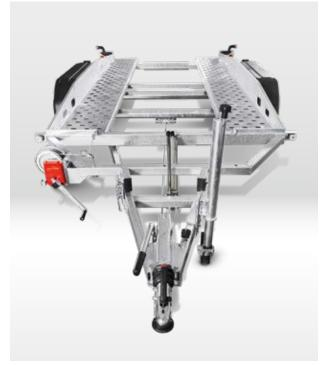
V-drawbar & coupling Optimum driving stability with the robust, bolted V-drawbar (except UT-AL 2515/75) and therefore easily exchangeable.
