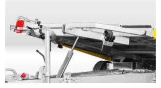
**Upper bridge** High load capacity due to hot-dip galvanised, solid upper bridge with cable winch and winch block as well as welded running rails (AT and AH series).
