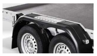
Alu checker plate on fenders for safe access to the mudguards without slipping (only AT- and UT-ST models)
