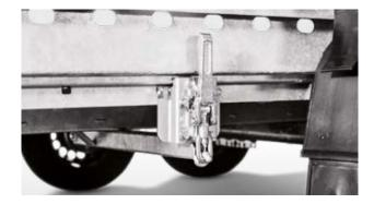
**Clamping locks** The drive-on rails are optimally secured by clamping locks and guarantee pleasantly smooth travel.
