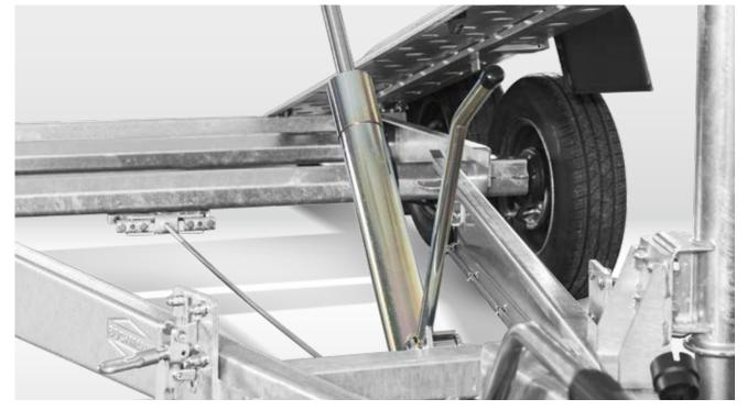
**Hydraulic, maintenance-free safety lifting system** for safe loading and unloading.
