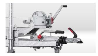
**Mechanical cable winch with winch block** for convenient and safe loading and unloading.
