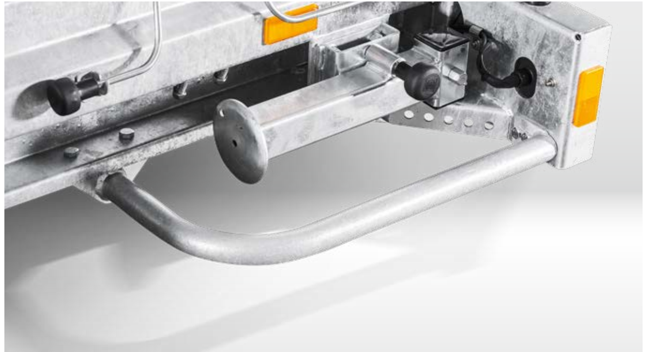
Protection bar The bar protects and supports the light box against side impact and deformation (illustration shows accessories: Telescopic crank support).
