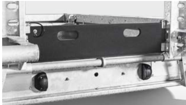
Slot-in board for safe closure of the loading area (AS models only).
