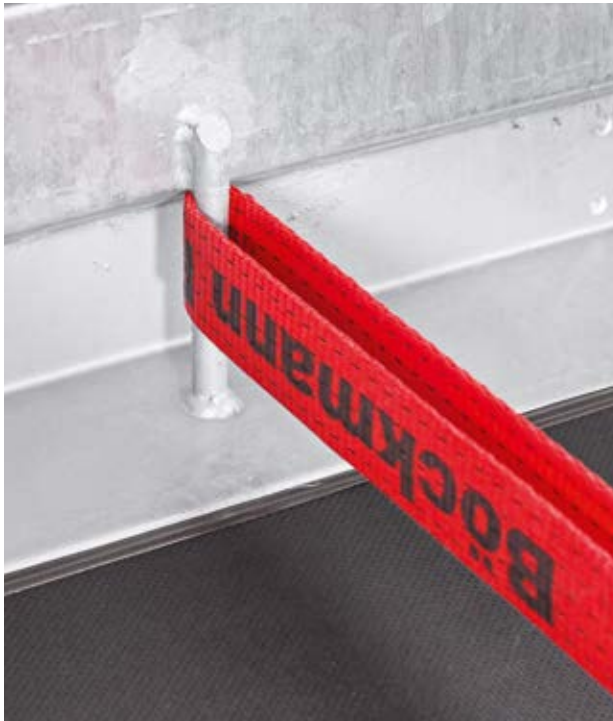
Lashing strips integrated into the side wall Up to seven lashing strips per side (model BT-ST 4019) integrated into the side wall (maximum tractive force up to 1000 daN).
