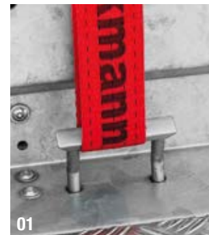
Additional rattle-free lashing brackets for securing the load during transport, available for BT-ST (01) and MH-AL (02) (maximum tractive force up to 500 daN).
