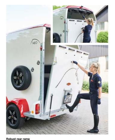
with integrated lifting device for easy opening of the rear ramp, additionally with sturdy double step.
