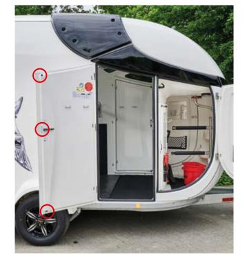
**Optimum closure** with the 3-point door lock and rubber seal.
