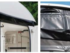
Protection against rain provided by the rain gutters above the doors and also in the rear area.
