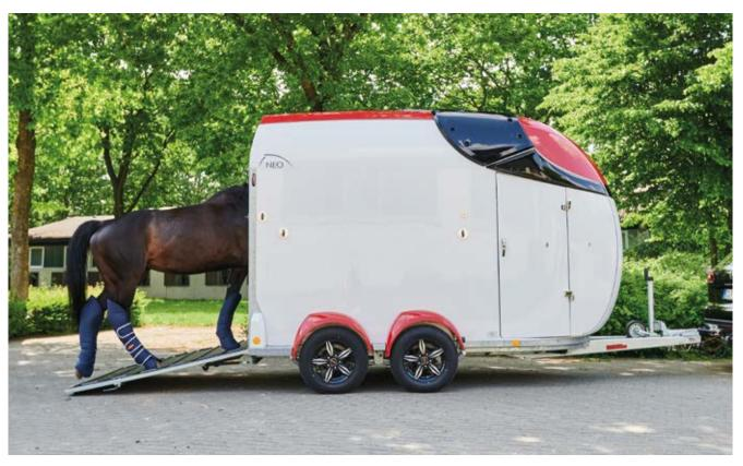
**Higher payload** due to the 2700 kg total weight as a standard feature instead of 2000 kg.
